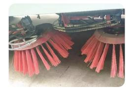
The road sweeper is equipped with a spray dust suppression device and a high-power dust suction motor that can effectively clean the dust.
